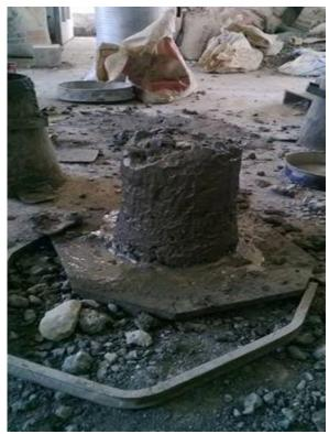
Fig 5.1(a) Slump Test of CS
