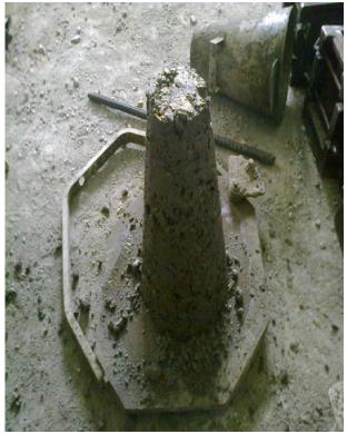
Fig 5.1(b) Slump Test of PRS
